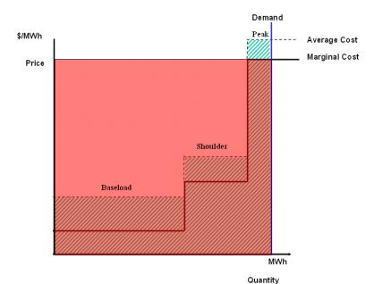
Figure 14: In the uniform-price auction used in U.S. RTO markets, all dispatched generation is paid based on the bid of the marginal generator (in this case, the peaking unit). The total generation cost of serving the load is equal to the amount of load served times the market-clearing price (the shaded box). Source: L. Lave, J. Apt, & S. Blumsack, Rethinking Elec. Deregulation, 17 ELECTRICITY JOURNAL 11 (2004).
