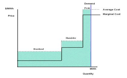
Figure 13: Under regulation, compensation for generators was based on the average cost of each plant. In this example, there are baseload, shoulder, and peaking plants. The total generation cost of serving the load is given by the shaded area under the average cost curve. Source: L. Lave, J. Apt, & S. Blumsack, Rethinking Electricity Deregulation, 17 ELECTRICITY JOURNAL 11 (2004).
