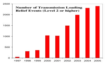
Figure 16: Number of transmission load relief events (level 2 or higher). Source: NERC.
