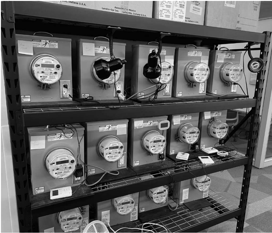
“Ping” testing devices (attached to middle row of smart meter bank) in operation and on display at SMUD’s offices.
